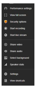
**Performance Settings:** Provides a smoother conference experience by reducing the image/sound quality in calls with insufficient bandwidth. The system performs performance settings automatically in the background under normal conditions. This menu should be used when adjustment is required by the user. If best performance is selected the videos will be disabled. (only speech)
